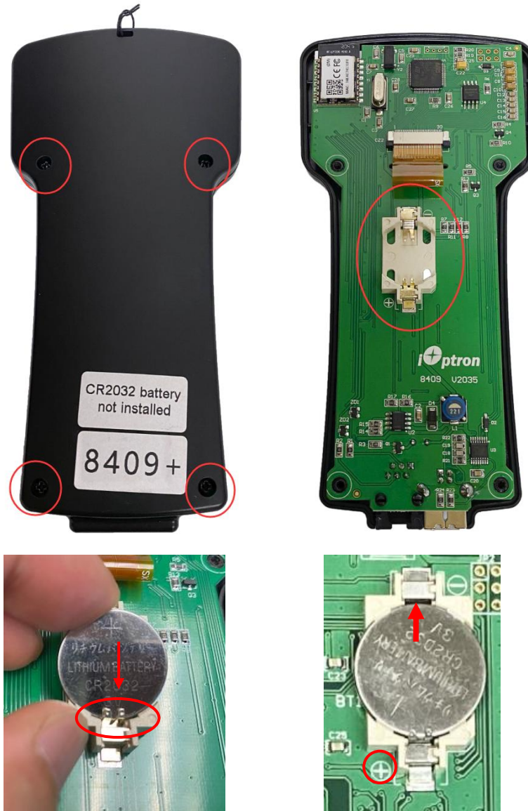
Figure 8. Install a CR2032 battery
