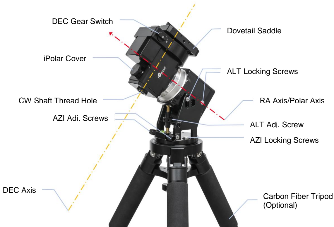
Figure 1. HEM27 mount assembly
