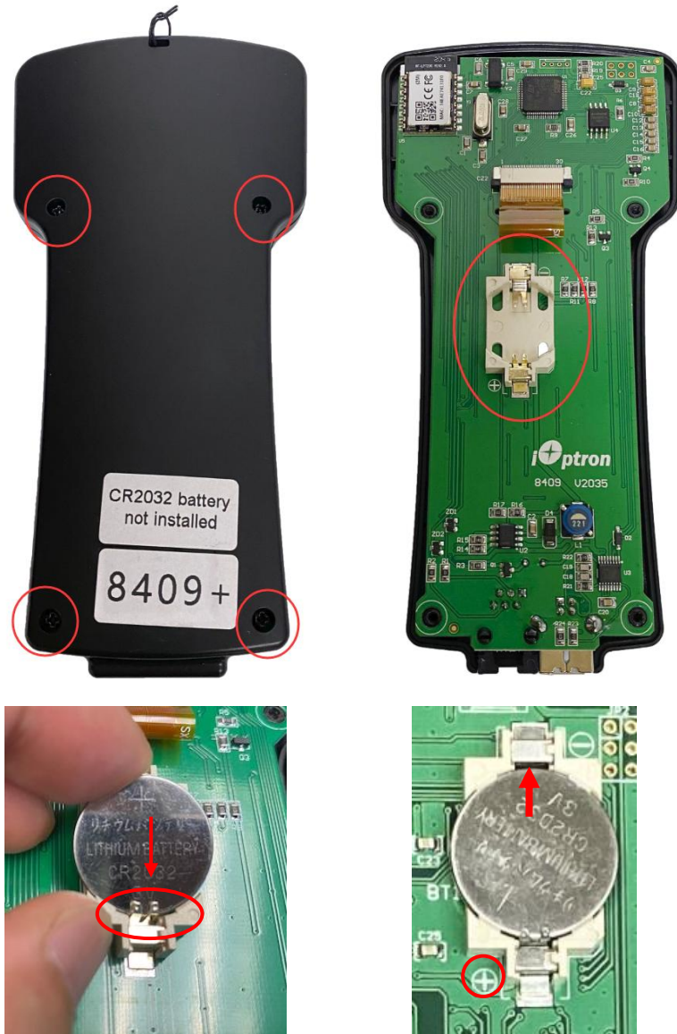
Figure 8. Install a CR2032 battery
