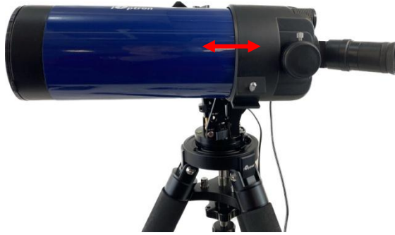
Figure 14 Balance the mount in DEC
