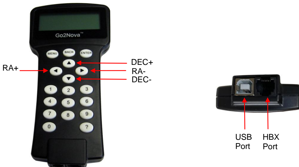
Figure 3. Go2Nova ® 8409 hand controller
