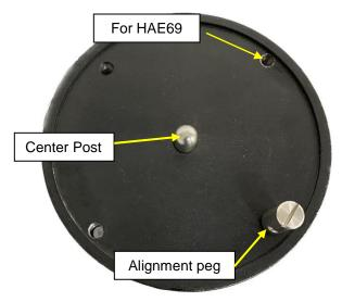
3. Attach mount head: Retract the 2X Azimuth (Azi) Adjustment Screws from both sides to leave ample space for the alignment peg to be fitted in between the 2X Azi Adjustment Screws.
