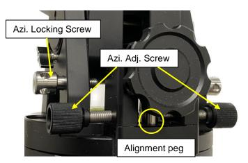
Remove Azi Locking Screws from the mount altitude arm. Secure the mount head by tightening the Azi Locking Screws into the M8 holes on the tripod. There is an Allen wrench stored on the mount base for tightening the screws.
