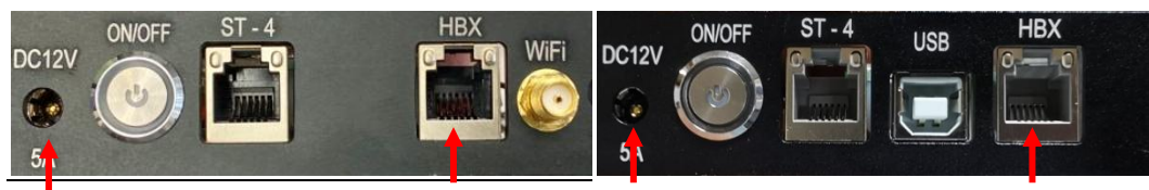
Figure 28. DC12V power and HBX port on mount base
