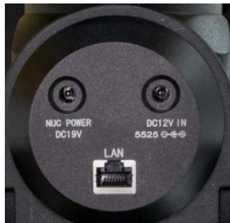
Figure 12. Ports on the rear end of RA axle
