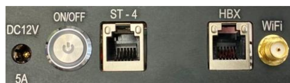
Figure 5. Ports on a CEM70G mount base
