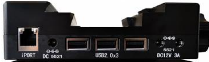
Figure 3. Ports on CEM70 dovetail saddle
