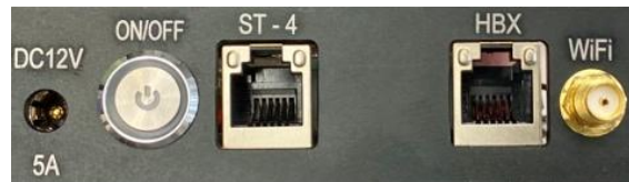
Figure 8. Ports on a CEM70W/CEM70WEC/CEM70EC2 mount base
