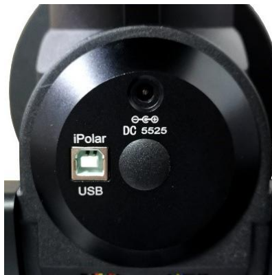
Figure 4. iPolar/USB and DC input on the rear end of RA axle
