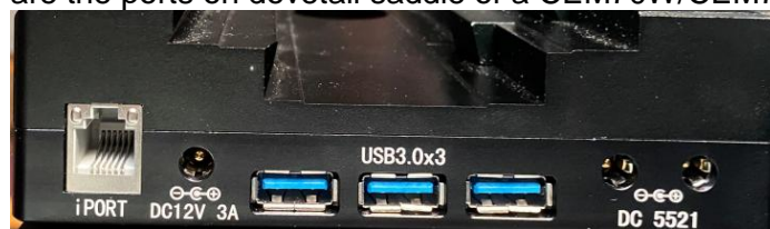
Figure 10. Ports on CEM70W/CEM70WEC/CEM70EC2 dovetail saddle
