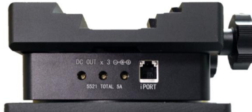
Figure 13. Cable/Ports connection of a CEM70-NUC
