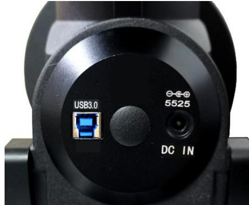
Figure 6. DC input on the rear end of RA axle
