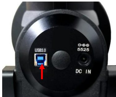
Figure 30. Connect CEM70G iPolar to a computer
