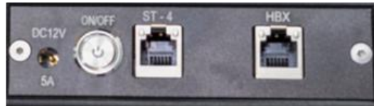
Figure 11. Ports on a CEM70-NUC mount base
