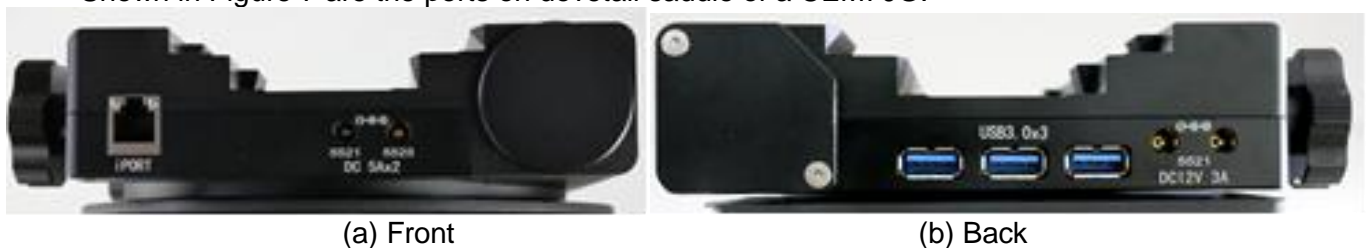
Figure 7. Ports on CEM70G dovetail saddle
