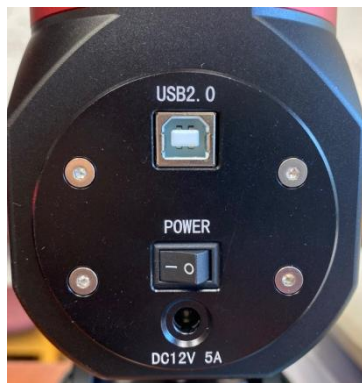
Figure 7. CEM40G Power Panel on Rear of RA axis
