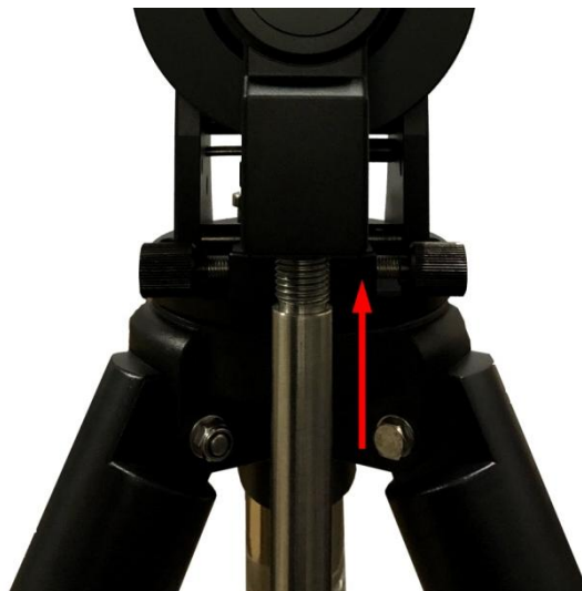
Figure 21. Install CW shaft
