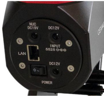
Figure 9. CEM40-NUC Input Panel on Rear of RA axis
