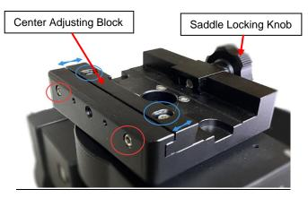
8. Balance payload: After attaching the scope and accessories, the mount head assembly must be balanced in both DEC and RA axes to ensure minimum stresses on the mount driving mechanism.
