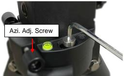
Level the mount by adjusting the tripod legs. Use the build-in Bubble Level Indicator or an external leveler for this purpose.
