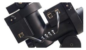
Connect the Go2Nova<sup>®</sup> 8409 Hand Controller to the **HBX** port on the main unit. Plug in a 12V DC power supply to the **DC12V IN** socket next to the **HBX** port, not the DC12V OUT next to GUIDE port.
