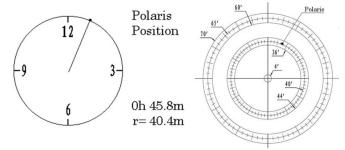
(3) Use the Azimuth and Latitude Adj. Knobs to adjust the mount in both directions and put the Polaris in the location on the Polar Scope Dial (same as indicated on the HC LCD), as shown in the right side of the above figures.
