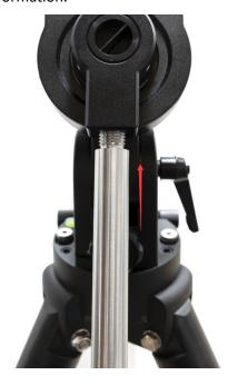
6. <u>Install counterweight</u>: Before putting on CW, make sure the mount is at its zero position, i.e., CW shaft points to the ground. **Insert Allen wrench to lock the RA axle** and disengage the R.A. Gear Switch to set the R.A. axis free before loading the CW. Remove the CW
