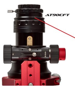
The 90CFT and 90EDX field flattener or the reducer/field flattener threads onto the camera angle adjuster that is attached to your focuser. Unthread\* the 2" eyepiece/accessory holder at the end of your focuser as well as the thin knurled black ring. Then simply thread your reducer/field flattener right into your camera angle adjuster.
