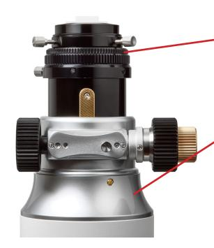
The EDT reducer/field flattener threads onto the camera angle adjuster that is attached to your focuser. Unthread the 2" eye-piece/accessory holder at the end of your focuser as well as the thin knurled black ring. Then simply thread your reducer/field flattener right into your camera angle adjuster.
