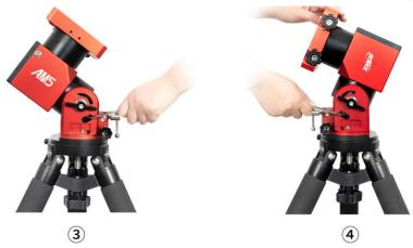
Manipulate the equatorial mount to slide and adjust the "altitude fine-tuning knob," allowing the hex screw to slide to the bottom end of the hole's slide rail, with the scale screw indicating at the 90° position. At the same time, expose the hex screw and retighten the hex screws on both sides (Note: After adjusting the gear position, be sure to tighten the gear screws firmly, otherwise the equipment may become loose and the gear adjustment function can be easily damaged).
