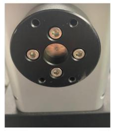
4. Release 4 screws on saddle adapter. remove the adapter and rotate it 90 degree. Re-install the screws and tighten them.
