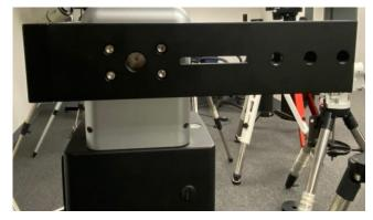
7. Thread in CW shaft in to one of three holes on the long bino adapter bar. Usually use the lowest one.
