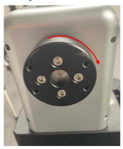
You have to rotate the saddle adapter itself, not by releasing the locking knob to rotate it wth the mount ALT axle.
