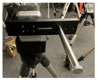
8. Install counterweight first. You may release the mount ALT locking knob to set the CW at the lowest position. Then mount the bino onto included dovetail plate. Or you may use your own adapter first then attach to bino dovetail plate. Slide the dovetail plate into the bino dovetail saddle. Make sure that the STOPPER on the play is on top when the mount is at Zero Position. It will prevent the scope slide out from the saddle accidently.
