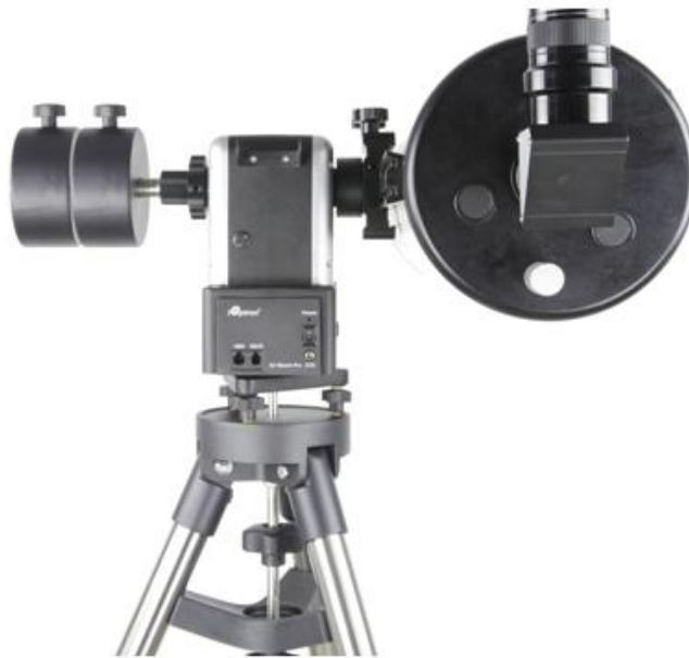
Figure 12 Heavy/large scope with two CWs
