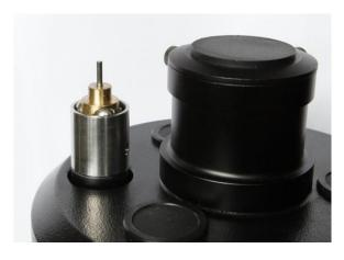
2. Pull the eFocuser out from the cover by remove three screws.
