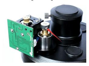
Wrap the belt on motor shaft first. The put it onto the eFocuser pulley. You may turn the pulley while install the belt. Adjust the motor mounting screws to adjust the belt tension if needed.
