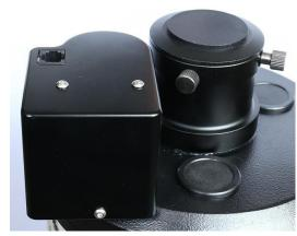
7. Connect the eFocuser to the mount use supplied 6P6C cable (same as the hand controller cable.) One end to the port on the eFocuser. The other end to the PORT on an iOptron mount.
