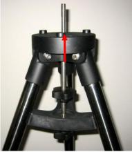
4. Release three locking screws located at the bottom of the MiniPier body. Put the Base Flange onto the tripod head. Using three M10 hex head screws to secure the base flange.
