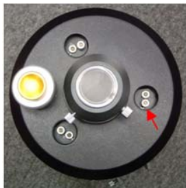
Figure 7a. First, turn the push screw counterclockwise a small amount, no more than a \frac{1}{4} turn. (Note: actual selected alignment screw will vary.)
