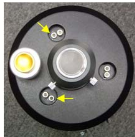
Figure 7c. Locate the pull screws in the other two screw sets and turn them counterclockwise no more than \frac{1}{4} turn.
