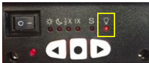
Figure 23 Polar scope LED intensity adjustment
