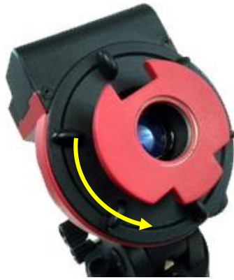
Figure 22. Adjust polar scope position if needed
